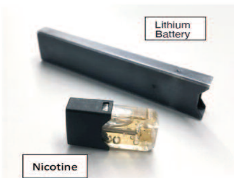
An e-cigarette showing the portions that contain the two hazards.
